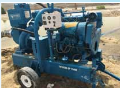
Dewatering Pumpset with Kirloskar engine in operation
