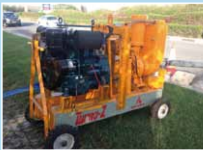
Dewatering Pumpset with Kirloskar engine in operation at a site in Dubai
