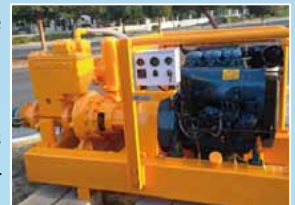
Dewatering Pumpset with Kirloskar engine in operation at a site in Dubai
